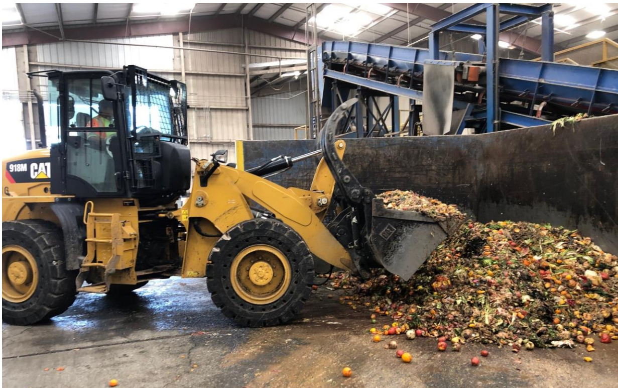
Figure 2. After an initial screening for contaminants on the MSS tipping floor, food scraps are loaded onto a conveyor belt for additional removal of contaminants. Source: MSS.
