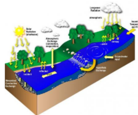
Figure 1. Major heat flux processes in streams. Click diagram to view a larger version.
