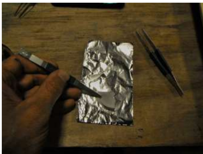
Figure 6. The proper method for folding the chlorophyll-a and AFDM filters.
