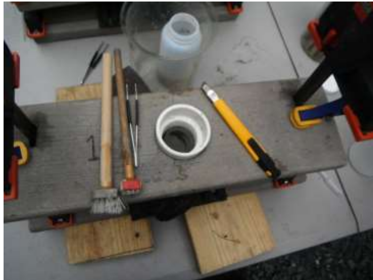
Figure 4. The Pennsylvania Epilithic Periphyton (PEP) Sampler with various tools used to sample algae from rock substrate. Rocks suited for periphyton scrubbing must be of size and shape to fit properly in the PEP sampler – large enough and flat enough for the sampler circular foam gasket to form a leak-proof seal around the area to be scrubbed.
