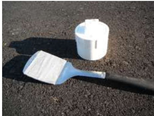
Figure 1 Silt/sand/gravel PVC and spatula sampling apparatus. This apparatus may consist of a section of capped 4 or 5-inch diameter PVC pipe and a kitchen spatula. The spatula must be large enough so that when it is slid under the PVC pipe it will prevent the loss of silt, sand, or gravel from the sample as it is pulled from the benthos.
