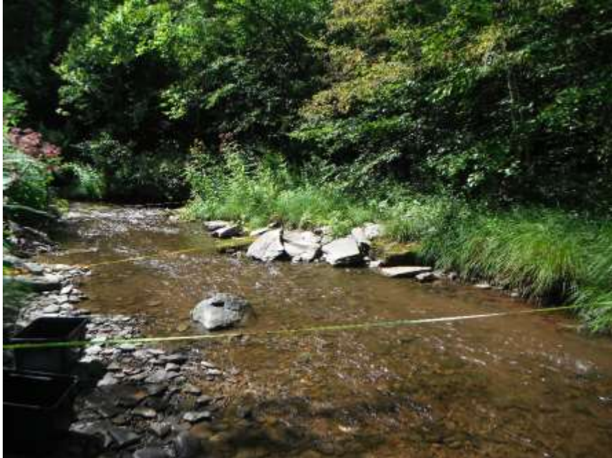
Figure 2. An example of a periphyton sample reach in a wadeable riffle-run stream. Three transect measuring tapes are pulled across the riffle section of the stream to facilitate random rock selections.
