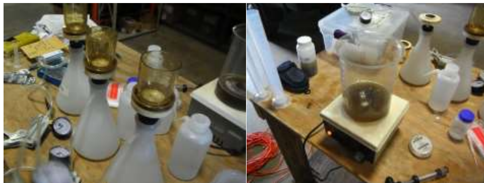
Figure 5. Vacuum-draw filtering devices on left and algal slurry beaker on a magnetic stirrer on the right.
