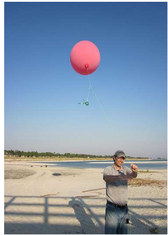
Helium balloon with digital camera attached
