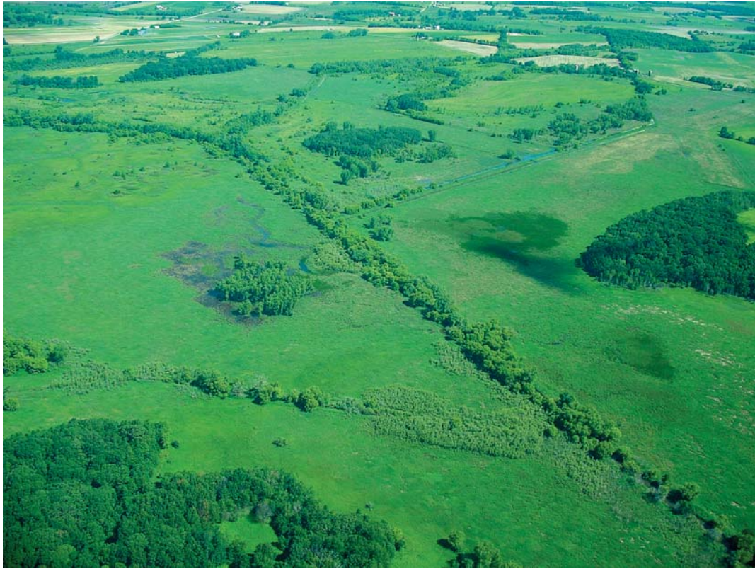
Figure 8. The straightened Mauneshia River (seen as the diagonal line of trees in the photograph) through Deansville Wildlife Area. Historic stream meanders can be seen on the left side of the existing channel. Water flowing down the channelized Mauneshia River rarely comes in contact with its floodplain and the surrounding wetland is thus hydrologically disconnected from the adjacent area. (Photograph, June 26, 2004.)
