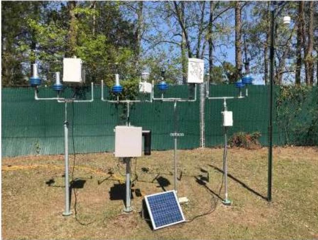
SPods (in blue) are fenceline monitoring devices developed by EPA to measure air pollutant plumes at an industrial facility. EPA scientists tested them at EPA's research campus in RTP, NC, alongside prototypes designed by commercial developers using the open source SPod technology.
